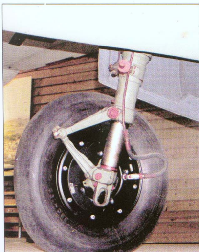
Bottom: Detail of the starboard main undercarriage wheel and the pressure hose of the hydraulically controlled brakes
