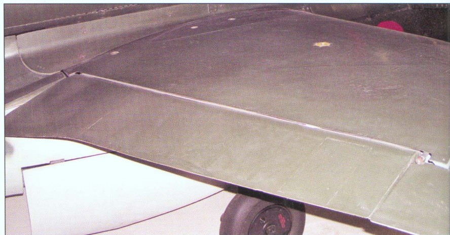
Above and below: Aerodynamic transition between the wing, fuselage and engine nacelle, below is shown for the starboard flap (Photo: M. Salajka)
