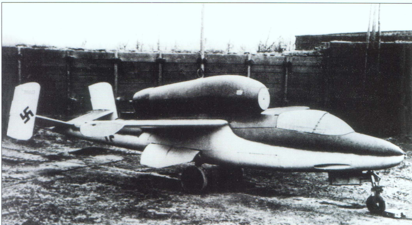
Heinkel He 162A-1 (?) vyrobený u Junkerse. Sériové letouny již dostaly silnější křídlo, včetně „ušť“ na koncích křídel • A Heinkel He 162A-1, manufactured by Junkers, armed with MK 108 cannons. The series built aircraft were equipped with strengthened wings, which included the “Lippisch ears” at the wingtips (P. Jarrett collection)
